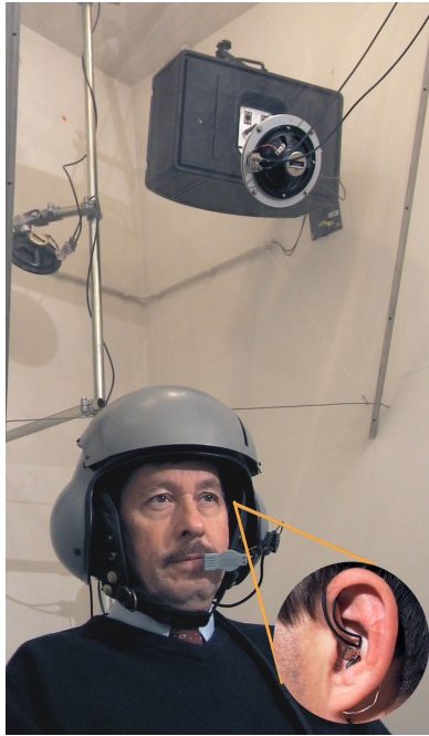
Figure 21. Subject positioned in a high-noise room and the mounting of the electret microphone near the entrance of the ear canal.
